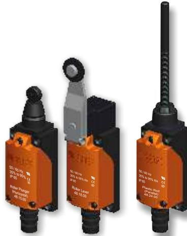
WERNER'S 48 series general purpose limit switches have a sturdy construction comparable to any limit switch. It uses a zinc die-cast body, a glass-weave reinforced plastic head, and a cover. The terminal cover also boasts excellent dust-proof and drip-proof capabilities.
